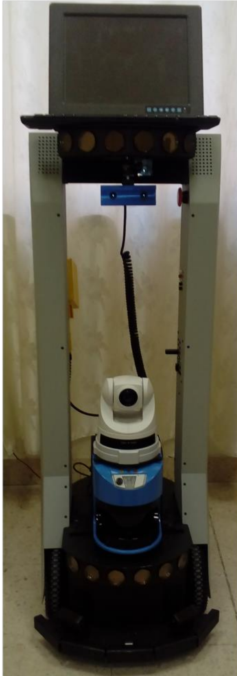
Figure 1 PeopleBot indoor robotic research platform equipped with SICK LMS-500 2D laser range finder, AXIS 214 PTZ network camera and a mobileRanger FPGA-accelerated C3D stereo camera.
