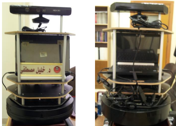
Figure 4: Turtlebot 2 mobile robot platform equipped with Kinect Xbox 360 RGB-D sensor
