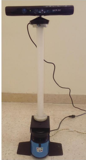
Figure 2 SICK LMS-100 2D LRF sensor and a Kinect Xbox 360 camera rigidly attached to each other to simulate an indoor mobile robot
